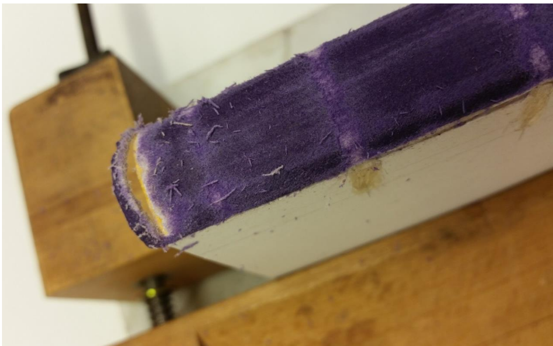
Sanding the leather spine lining to reveal the yellow endbands
