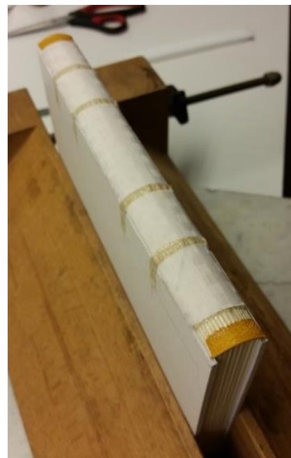
Left: Rounding and backing the spine of the sewn text block
