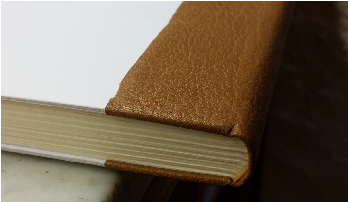
The pared leather glued to the spine of the book, with turn-ins visible around the endband
