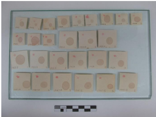
Figure 2: The samples of paper after lignin and alum testing. The big spots are to test for lignin and the small spots are to test for alum. Only one book, printed in 1944, contain lignin and all books contained alum.
