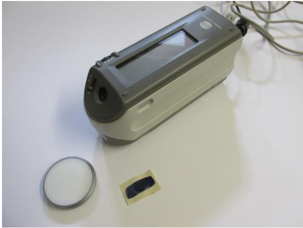
Figure 4: The Konica Minolta Colour Spectrophotometer, this is an analytical tool used to measure colour. The Spectrophotometer flashes a light on to the sample and with the information it receives it makes a unit measurement which signifies the location of the sample's colour on the CIE L*a*b* sphere. The CIE L*a*b* colour sphere holds all the colours and their varied hues in a round ball; it is used to measure the difference between two colours.
