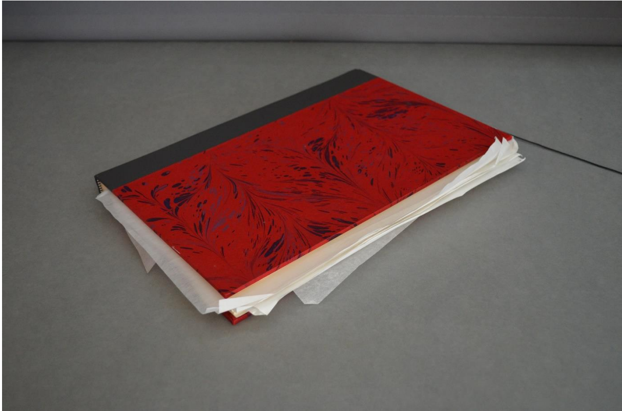
Figure 1: Side view of the book after 50 people had handled it. You can clearly see the dislodgement of the interleaves that have been placed in loosely
